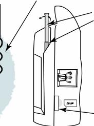
The broken piece of telescopic antenna must be unscrewed (by turning anti-clockwise) and removed from the silver base tube.
